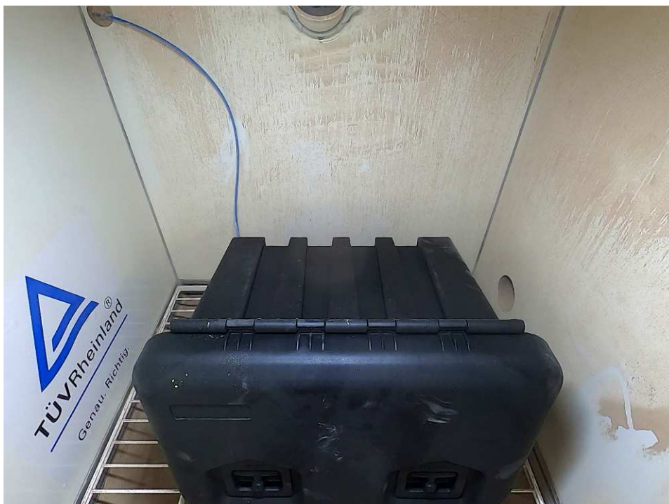
Bild 2: Muster in der Staubkammer / Picture 2: Sample in dust chamber
