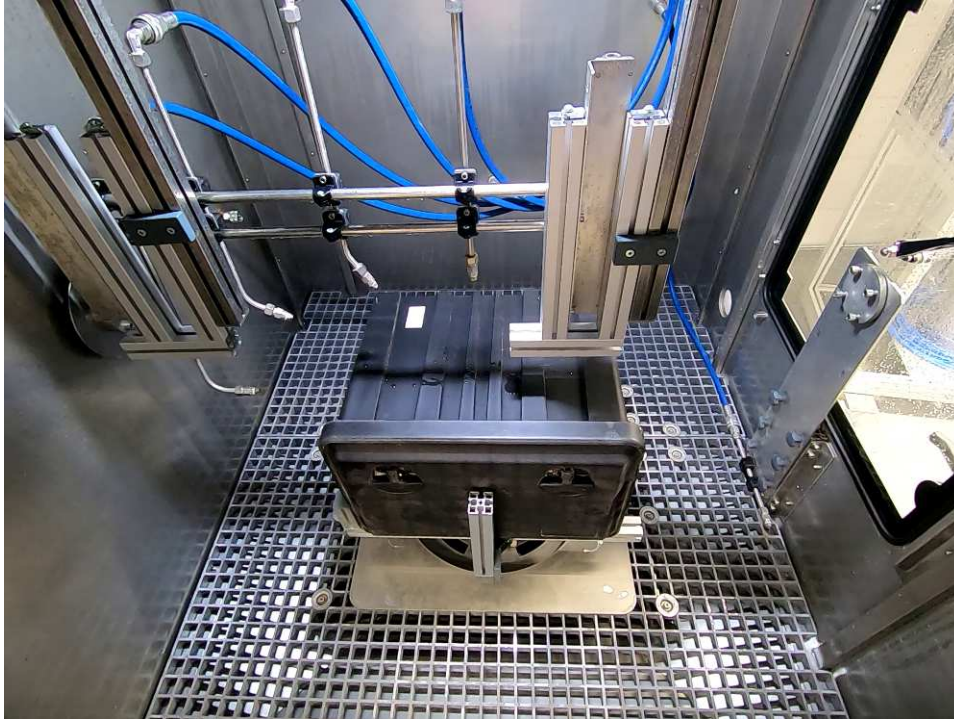
Bild 3: Muster in der Wasserkammer / Picture 3: Sample in spray water chamber
