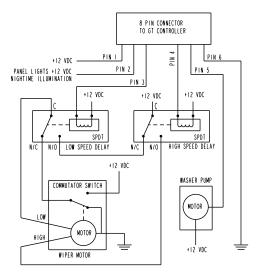
NOTE: ALL RELAY SWITCHING IS DONE ON THE LOW SIDE. OTHER SIDE OF RELAY CONNECTS TO +12 VDC.
